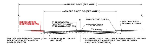
REINFORCED CONCRETE PAVEMENT
