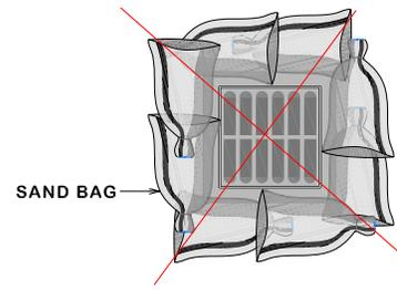
TEMPORARY DEVICES AROUND STORMS DRAINS ARE USED TO DETAIN AND/OR FILTER SEDIMENT-LADEN RUNOFF. THE PROTECTION ALLOWS SEDIMENT TO SETTLE PRIOR TO DISCHARGE INTO A STORM DRAIN INLET OR CATCH BASIN.
