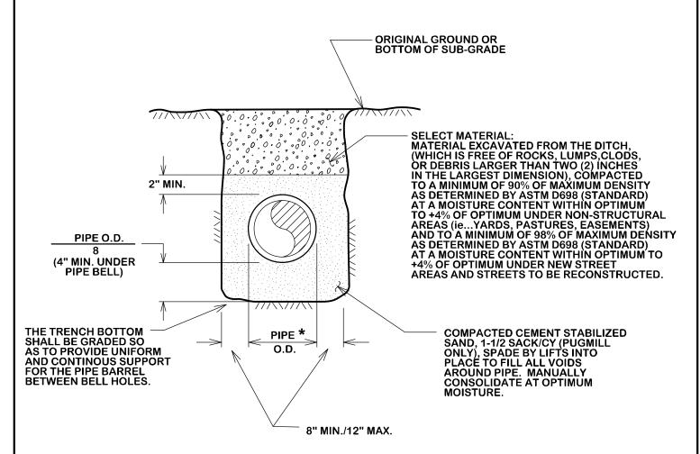
\* PE MUST DESIGN TRENCH DETAIL SITE SPECIFIC FOR HDPE PIPE.
